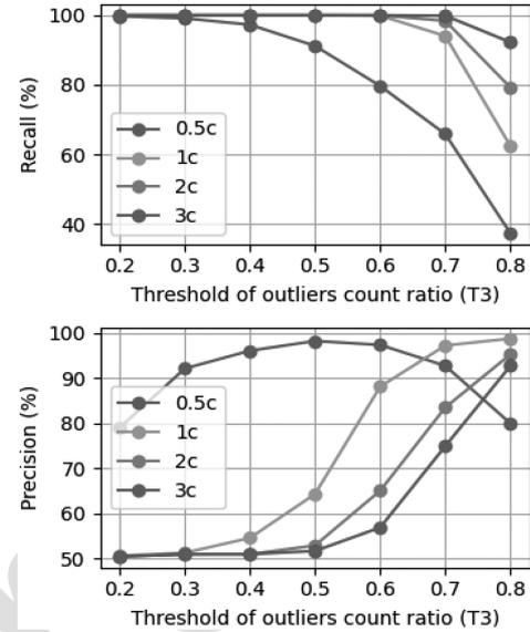
Fig. 3. Performance metric curves representing the effect of threshold  $T_3$  on RANSAC-based fault detection with different numbers of artificial cycle slips.
