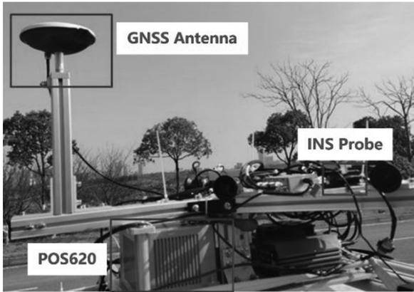
Fig. 6. Installation of the equipment used for the field land vehicle test.
