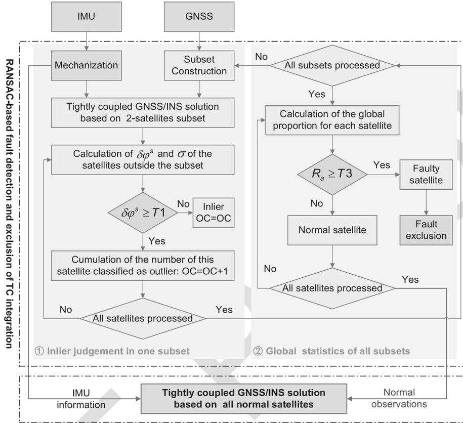
Fig. 2. Flow chart of RANSAC-based fault detection and exclusion of tightly coupled GNSS/INS integration.
