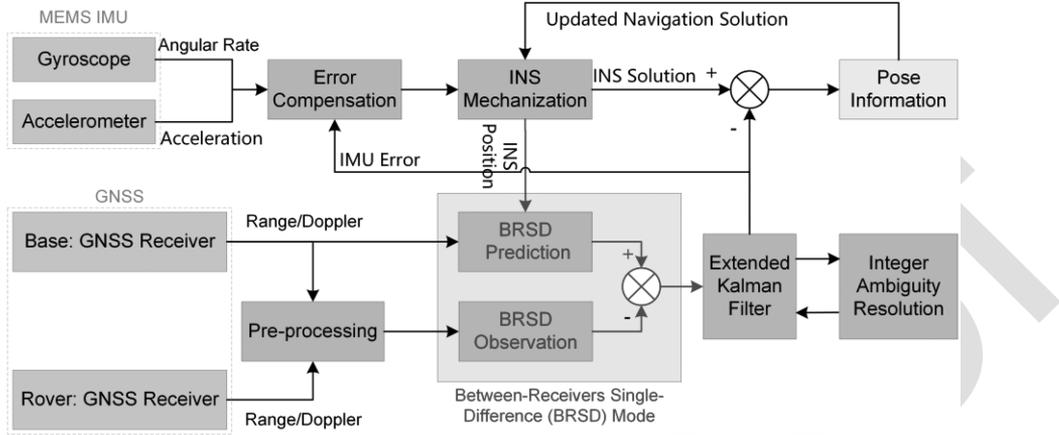
Fig. 1. Block diagram of tightly coupled GNSS RTK/INS integration based on a between-receiver single-difference model.
