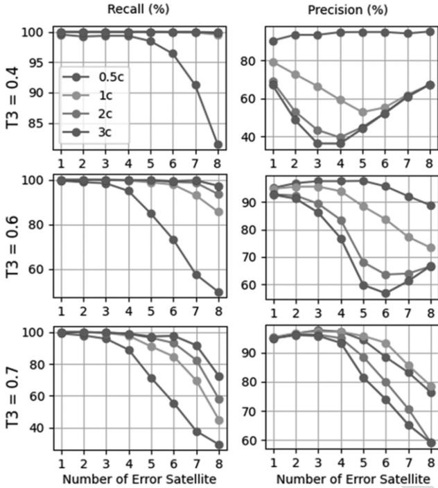
Fig. 4. Performance metrics curves representing the effect of the number of faulty satellites on the RANSAC-based fault detection with different numbers of artificial cycle slips.
