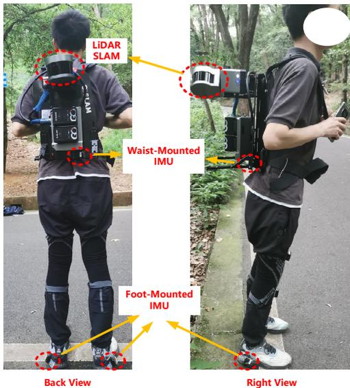
Fig. 4. The relative positional relationship between foot-mounted IMU, waist-mounted IMU, and LiDAR SLAM.
