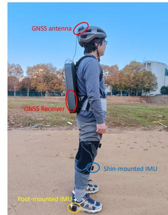
Fig. 7: The relative position of the experimental equipments on the human body.
